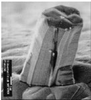
Subcontractor 'C' TO-220 unit at 7500X, 3634 hours exposure, precondition + 51C/85RH, unbiased. Whisker length = 9.3µ.
