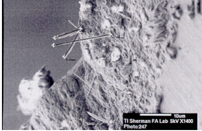
Subcontractor 'A' SOIC unit at 1400X, 3000 hours exposure, no precondition, bias + 51C/85RH. Whiskers with length = 8.0-17.7µ .
